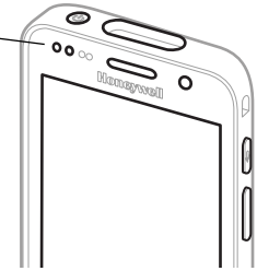
Battery Status LED
